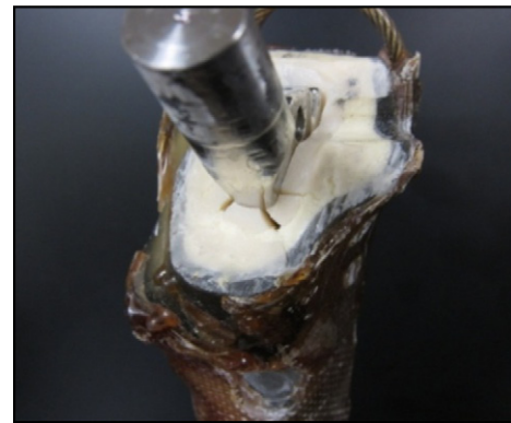
Figure 7. Photo of sample 3 showing the development of a cement fracture during loading 3. Multiple cracks are observed around the corners of the metallic stem.
